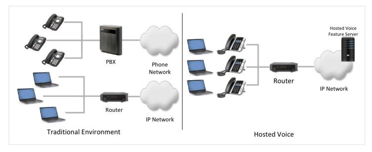
In a traditional environment, multiple connections are required to deliver voice and data, and multiple pieces of equipment are needed. With Hosted Voice, a single IP connection delivers everything you need for voice and data, including the phone system functionality.
